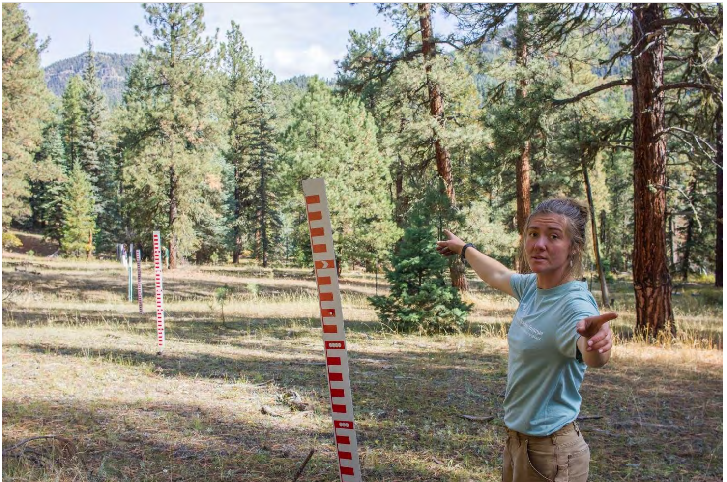
Lenka Duskocil, the water program research associate at Mountain Studies Institute, explains how the Jackson Mountain snowtopography site is designed to capture data on snow melt timing and pace along the edges of the clearing. (Reuben Schafir/Durango Herald)
