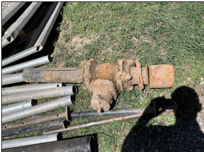
Distribution system isolation valve replacement
