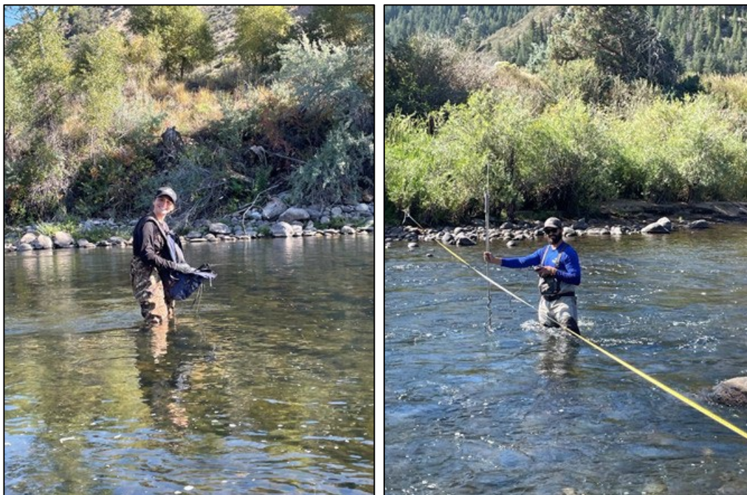
Flow measurement and water sampling during September water quality sampling event
